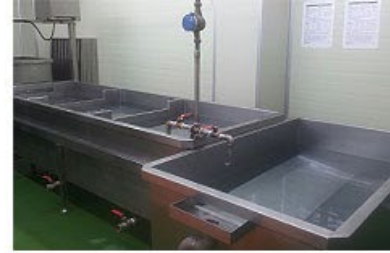
세척조 Washing tank
